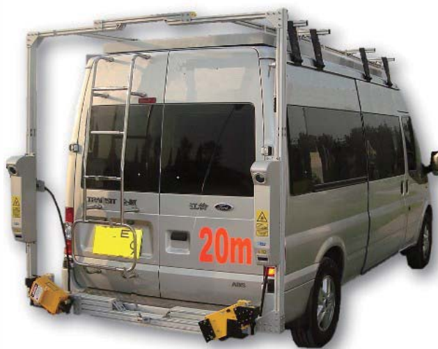
ROMDAS System with LRMS, Sub Meter GPS, High Resolution DMI and 2 Laser Profilometers.
